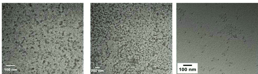
Figure 3. TEM pictures of brominated diblock copolymers left: Br-3 , middle: Br-5 , right: Br-4 .
